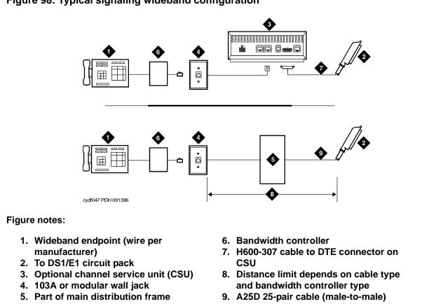
Figure 98: Typical signaling wideband configuration
